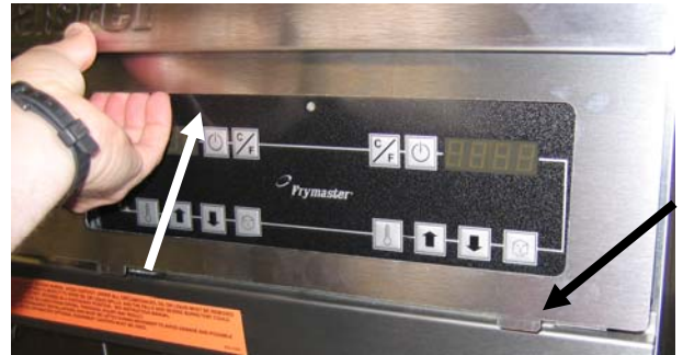
Figure 1: Slide the bezel up to disengage lower tabs.
